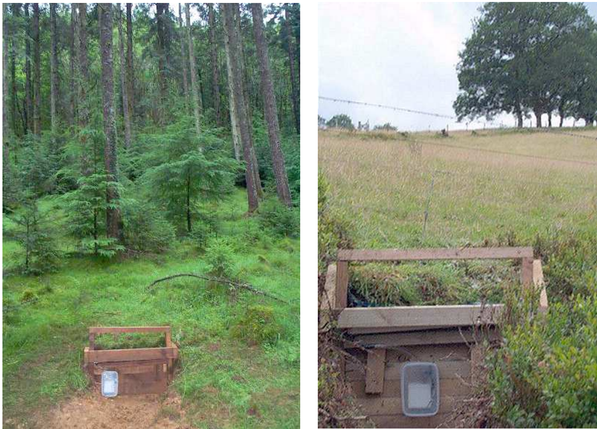
Figure 1.78: Surface runoff experiment, Hermon. (left) Site 1 beneath mature conifer plantation. (right) Site 3 beneath permanent grassland.
